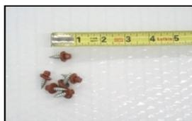
**Diaphragm screws** are 1-1/2" and have an outward tapered shank directly below the head. They are used to install roofing and siding with tip placed into a wood member beneath the steel sheeting.
