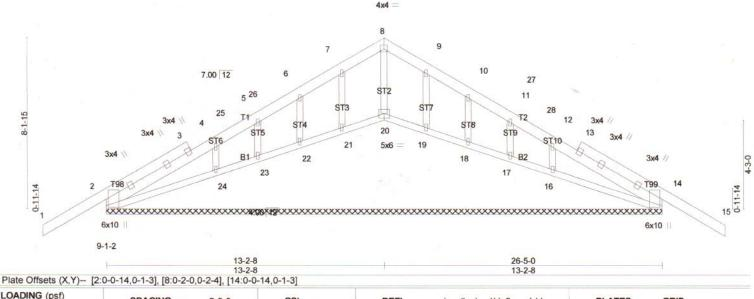
LOADING (psf) SPACING-2-0-0 CSI DEFL I/defl L/d **PLATES** GRIP TCLL Plate Grip DOL 1.15 TC 0.28 Vert(LL) -0.09 15 n/r 120 MT20 197/144 (Roof Snow=40.0) Lumber DOL 1.15 BC 0.13 Vert(TL) -0.11 15 n/r 90 TCDL 7.5 Rep Stress Incr YES WB 0.06 Horz(TL) 0.01 14 n/a n/a 0.0 \* BCLL Code IRC2009/TPI2007 Matrix-S Weight: 138 lb FT = 0% BCDL 7.5
